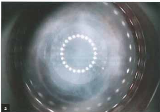
Light source for microscope consists of fluorescent diodes arranged in a circle.
